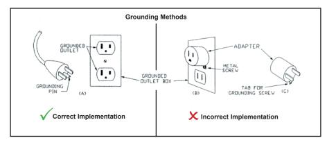
Improper connection of the equipment-grounding conductor can result in a risk of electric shock. Check with a qualified electrician or service person if you are in doubt as to whether the product is properly grounded. Do not modify the plug provided with the product - if it will not fit the outlet; have a proper outlet installed by a qualified electrician.
