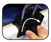
Firmly tighten the knob by turning clockwise to avoid slipping when in use.
