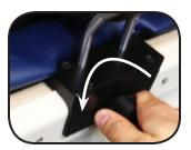
Loosen knob by turning counter-clockwise.
